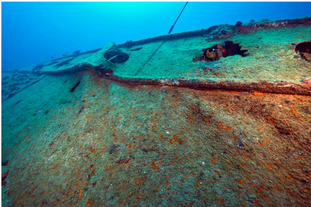
Figure 2. Hull buckling and warping is clearly visible in dive inspections after Cyclone Yasi's passage (Photograph: David Wachenfeld, Triggerfish Images).
